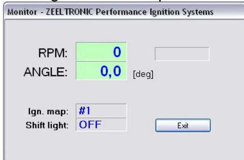
⇒ Monitor show engine revolution, ignition advance angle, selected ignition map, shift light status and rev limit activation.
